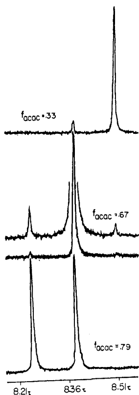
Figure 3.—Methyl proton resonance spectra for equilibrium mixtures of Ga(acac) 3 and Ga(hfac) 3 in benzene at 36°. Total solute molarity is 0.10 M. The two spectra shown for f_{\text{acac}} = 0.67 differ only in spectrum amplitude.
